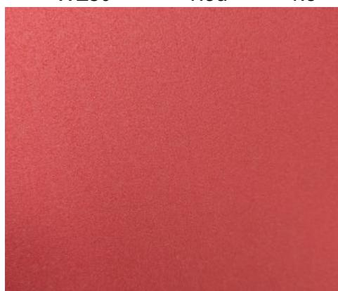
Zote foam is a crosslinked polyethylene with a low density. It is lightweight, latex free, non-toxic, and hypoallergenic. Other qualities include temperature resistance, and thermal conductivity.
